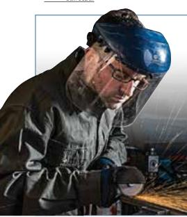
The Norton small diameter cut-off wheel line consists of Type 01/41 straight and Type 27/42 depressed center cut-off wheels from 1-1/2" to 9" diameters. These wheels come in ultra thin .035" for quick burn-free and burr-free cutting to .125" for more durable applications. All are reinforced for the demanding nature of portable cut-off.
