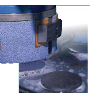
Surface grinding segments are generally used to grind flat stock or flat surfaces within a workpiece. The segment moves over the workpiece in a flat plane or vice versa. Applications can vary from heavy, rapid stock removal to precision tolerance operations.
