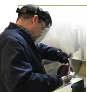
Made from non-woven synthetic fiber mesh, which is impregnated with abrasives and bound with resins, non-woven wheels are designed to create desired surface finish where little or no stock removal is required. Non-woven wheels have an open mesh construction that is waterproof, washable, conformable and non-loading.
