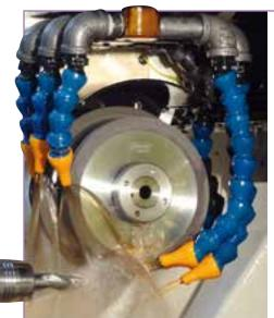
Norton Winter offers an extensive line of stock Diamond and cBN (cubic Boron Nitride) grinding products, including resin, vitrified, metal and MSL (metal single layer) bond offerings, under the "99" quality line. Premium, high-performance stock resin bond options are also available.
